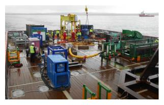
Figure 12 – Landing the export cable on deck
