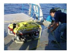
Figure 19 – Falcon ROV being prepared for deployment
