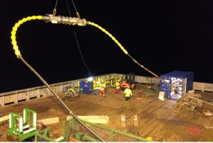
Figure 14 – Dry-mate being handled for deployment
