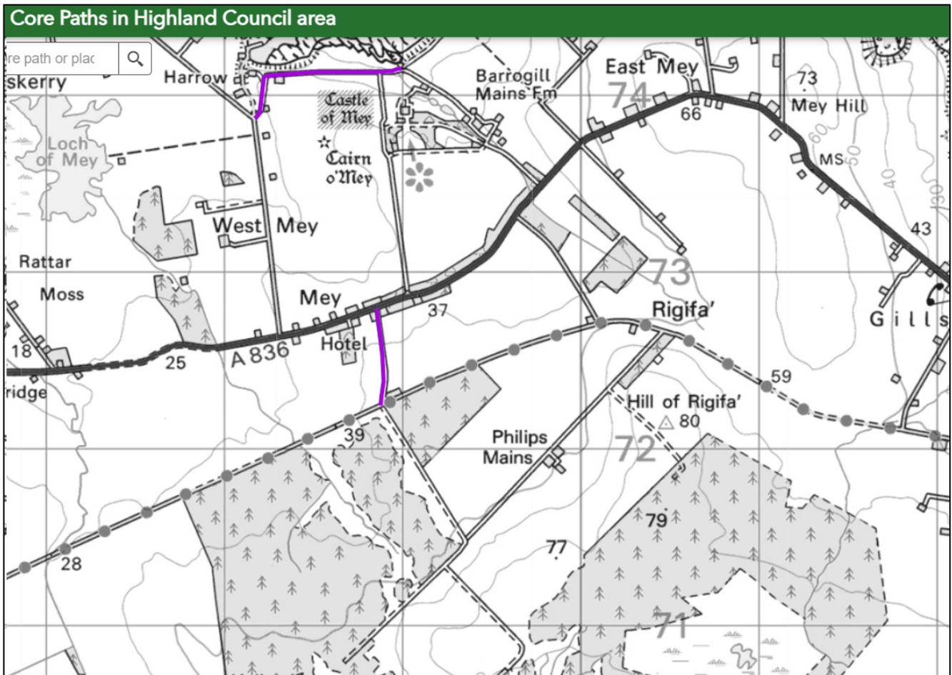
The Proposed Development area does not intrude on the Core Path alignment. To ensure that construction traffic does not affect users of the Core Path, the construction routing would not use the public road to the northwest of the Proposed Development site to access the A836.
